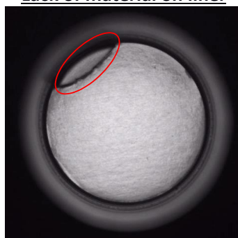
Lack of material on liner
